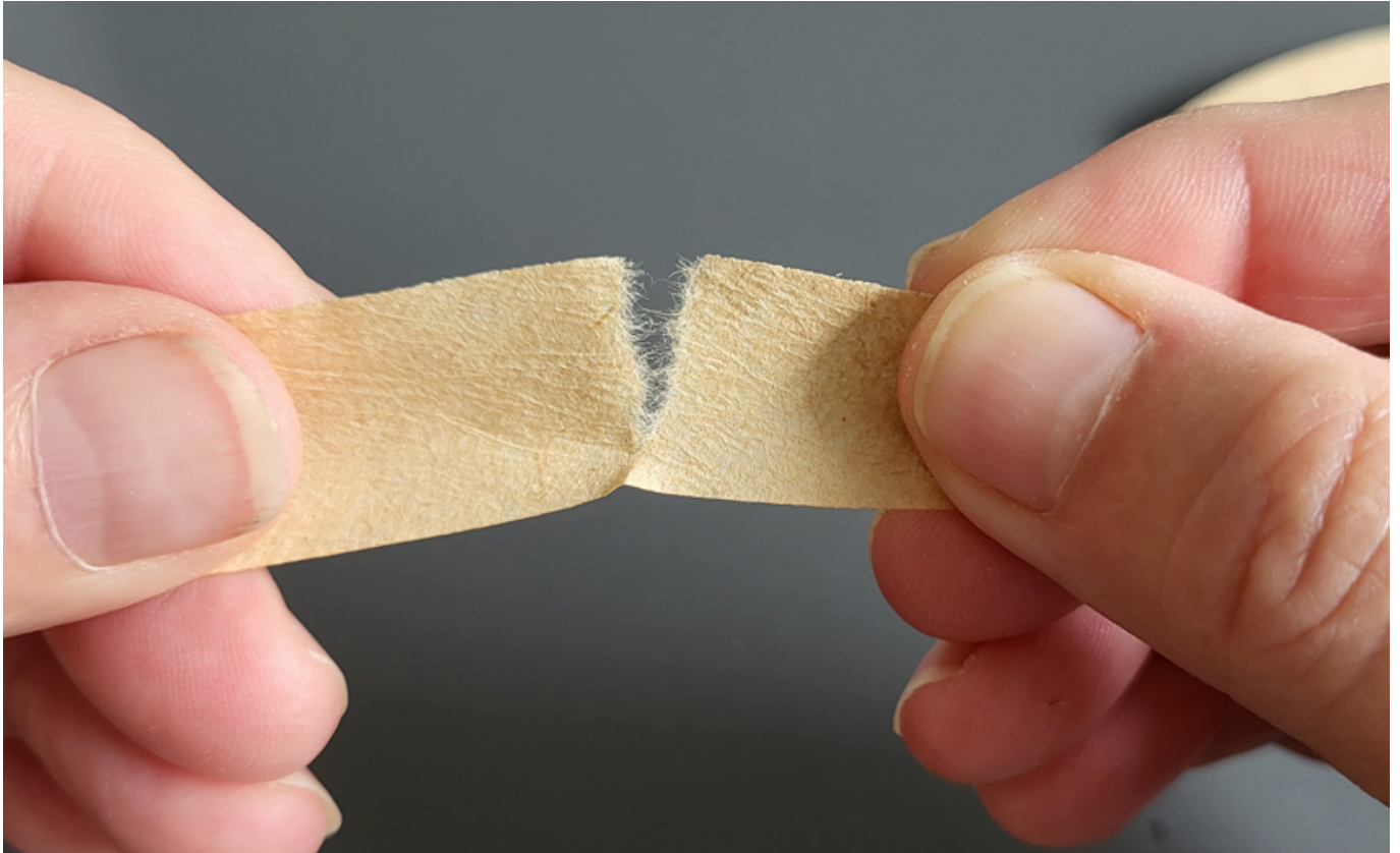
Fig. 4: To achieve the smallest layer thicknesses, it is necessary to tear the filter strips.
