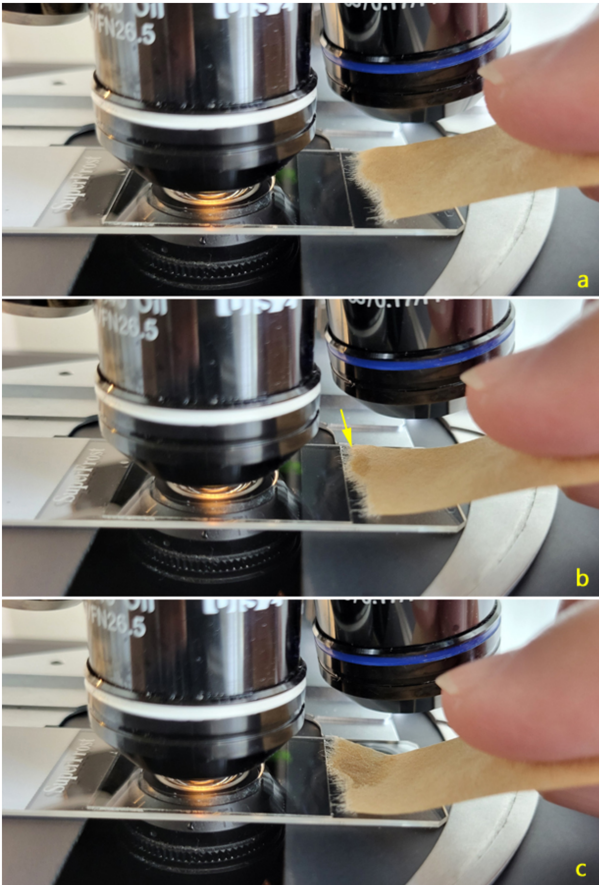
Fig. 5 a-c: The fine fibers of the torn strips extend to the water film under the coverslip. It may take a few seconds for the capillary effect to become visible (b,
