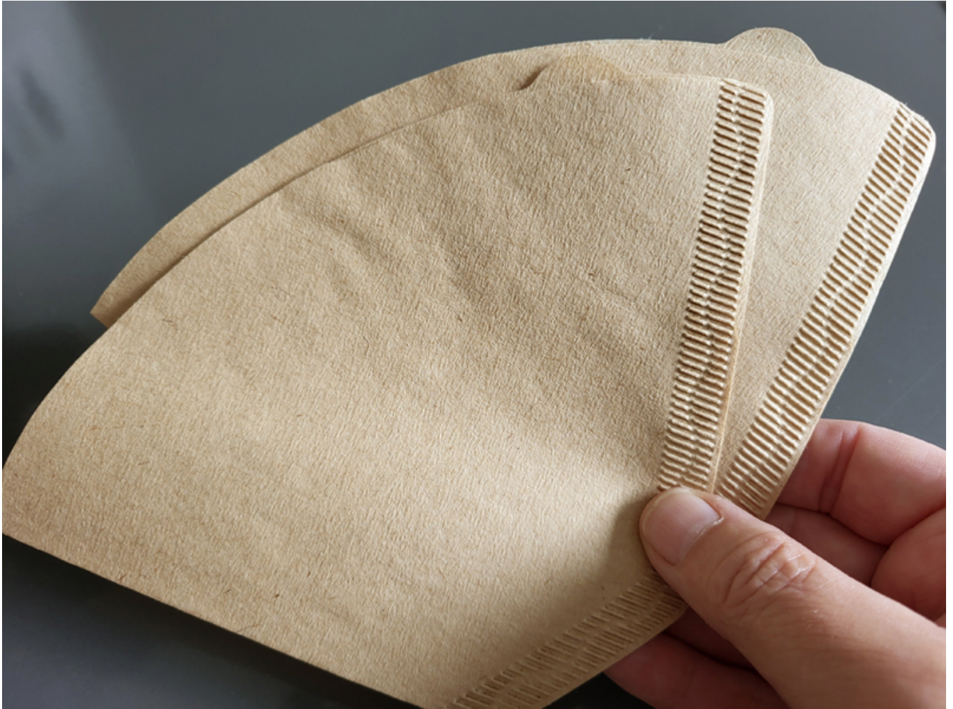
Fig. 1: Use of common coffee filters für adjustment of the layer thickness.
