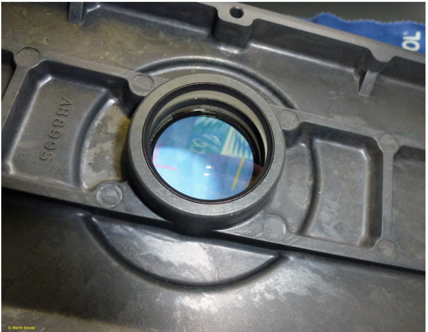
Fig. 10: The lens embedded in the base plate after cleaning with glass cleaner.
