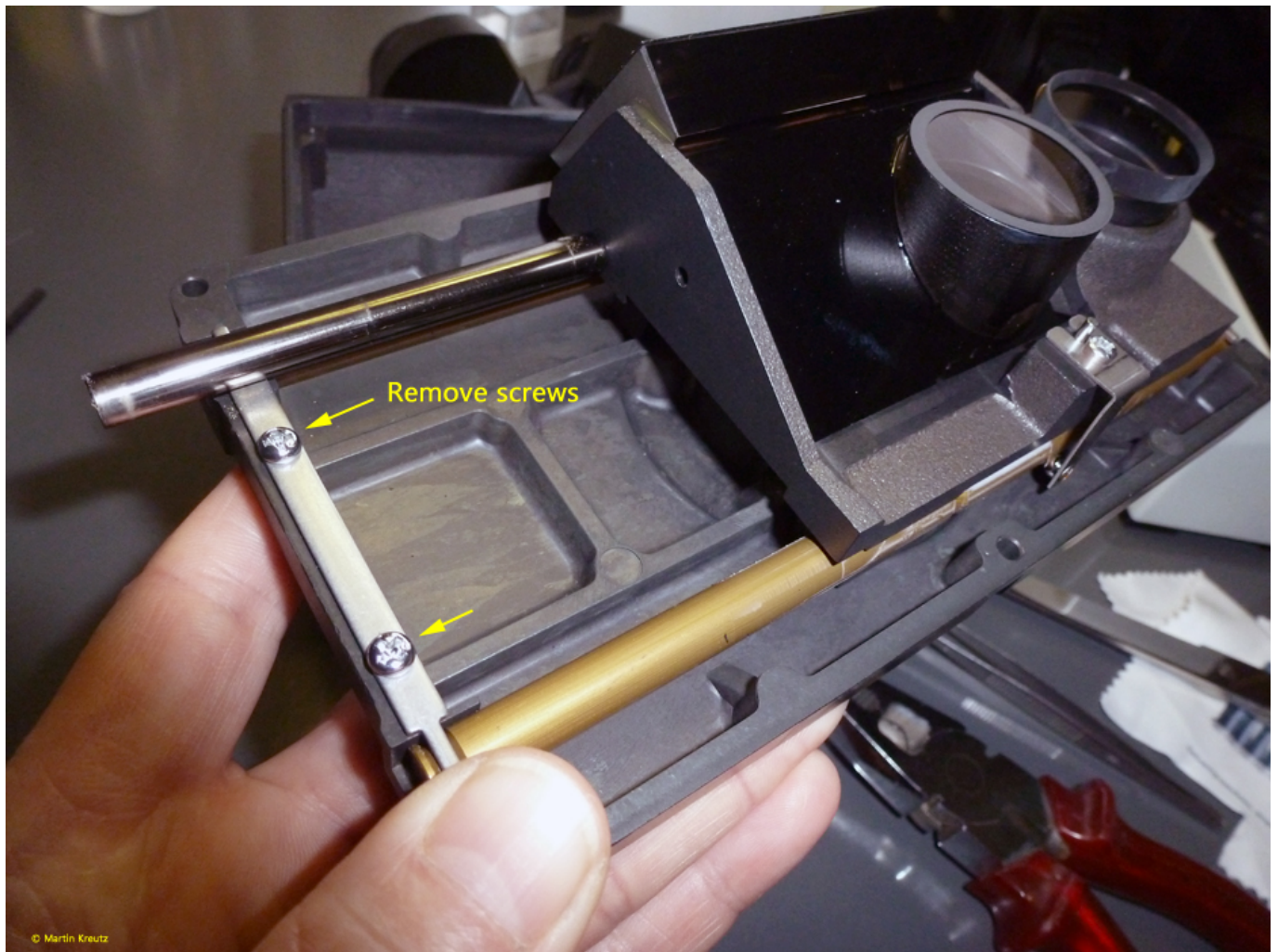
Fig. 6: Remove the screws of the fixing bracket on the left side.
