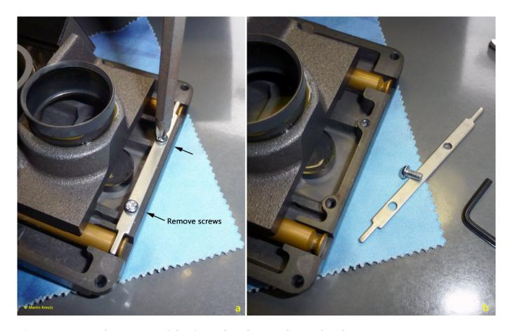
Fig. 7: Remove the screws of the fixing bracket on the rigth side.
