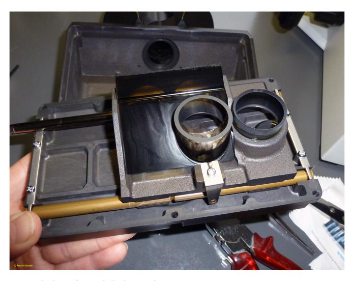
Fig. 5: The base plate with the beam splitter.
