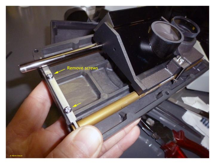
$\textbf{Fig. 6:} \ \ \text{Remove the screws of the fixing bracket on the left side}.$
