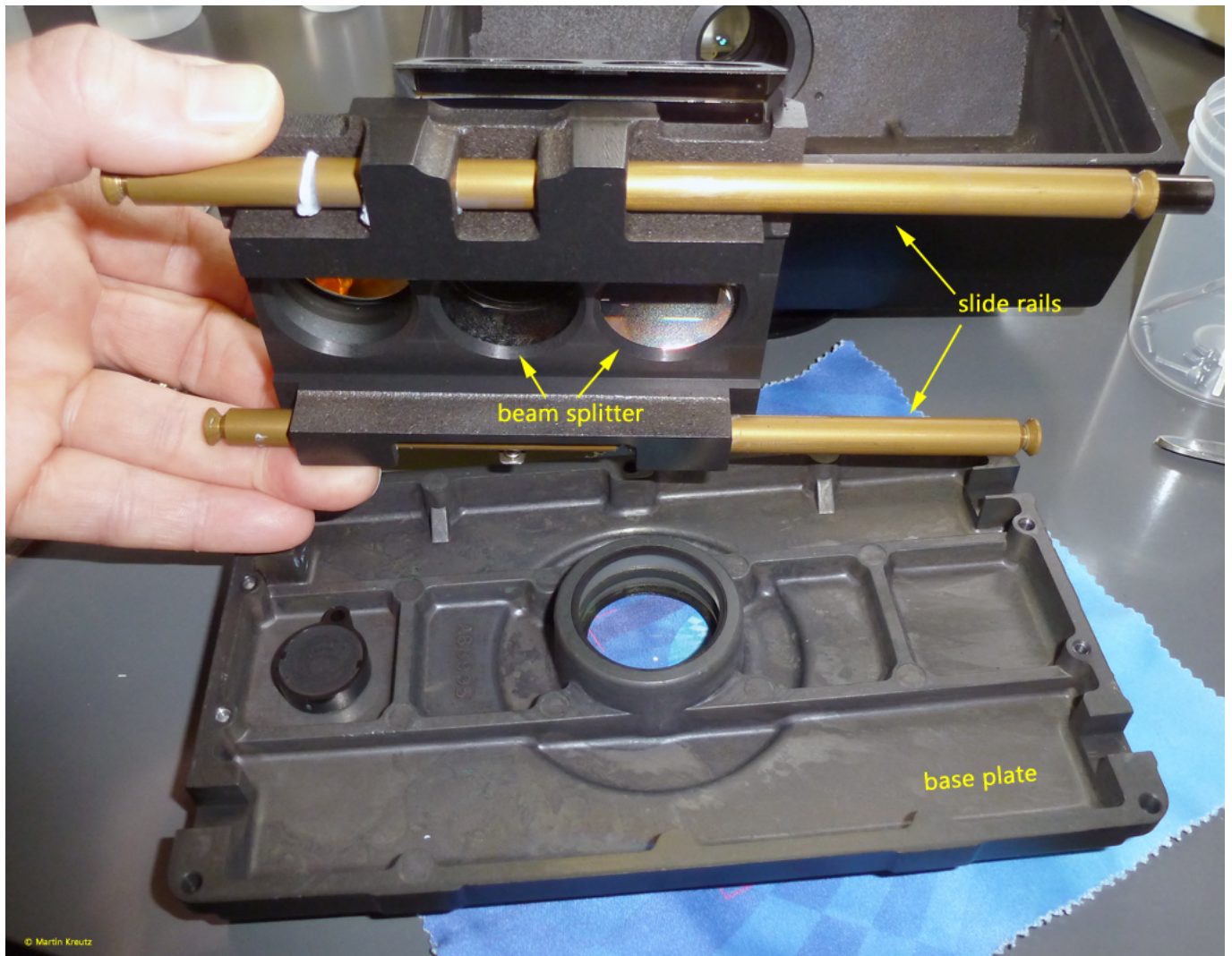
Fig. 8: The detached beam splitter from the base plate.
