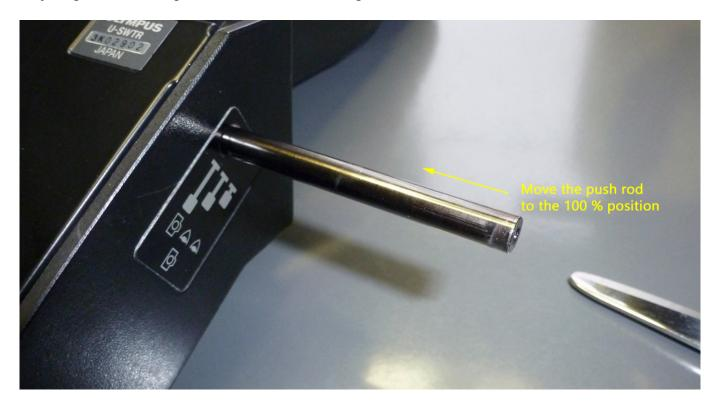
**Fig. 4:** Move the push rod to the 100% position.
