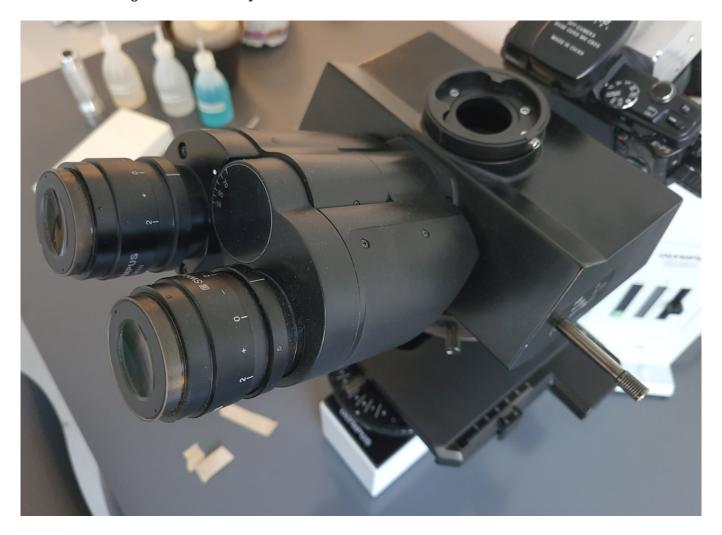
Fig. 1: The Olympus super widefield trinocular tubus U-TRSW.
