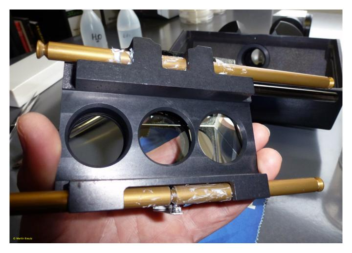
Fig. 9: The slide rails with new grease.
