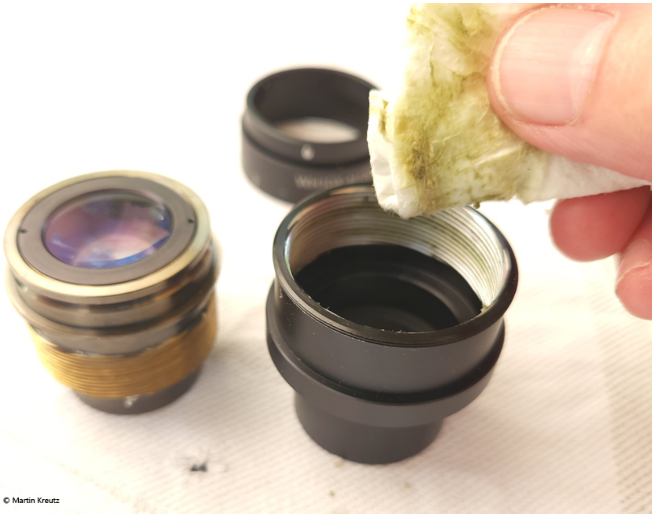
Fig. 7: Cleaning of the threads with spirit and cellulose.
