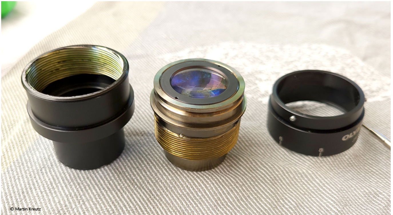
Fig. 6: Once the gun oil has dissolved the resinified grease, the brass sleeve can be unscrewed.
