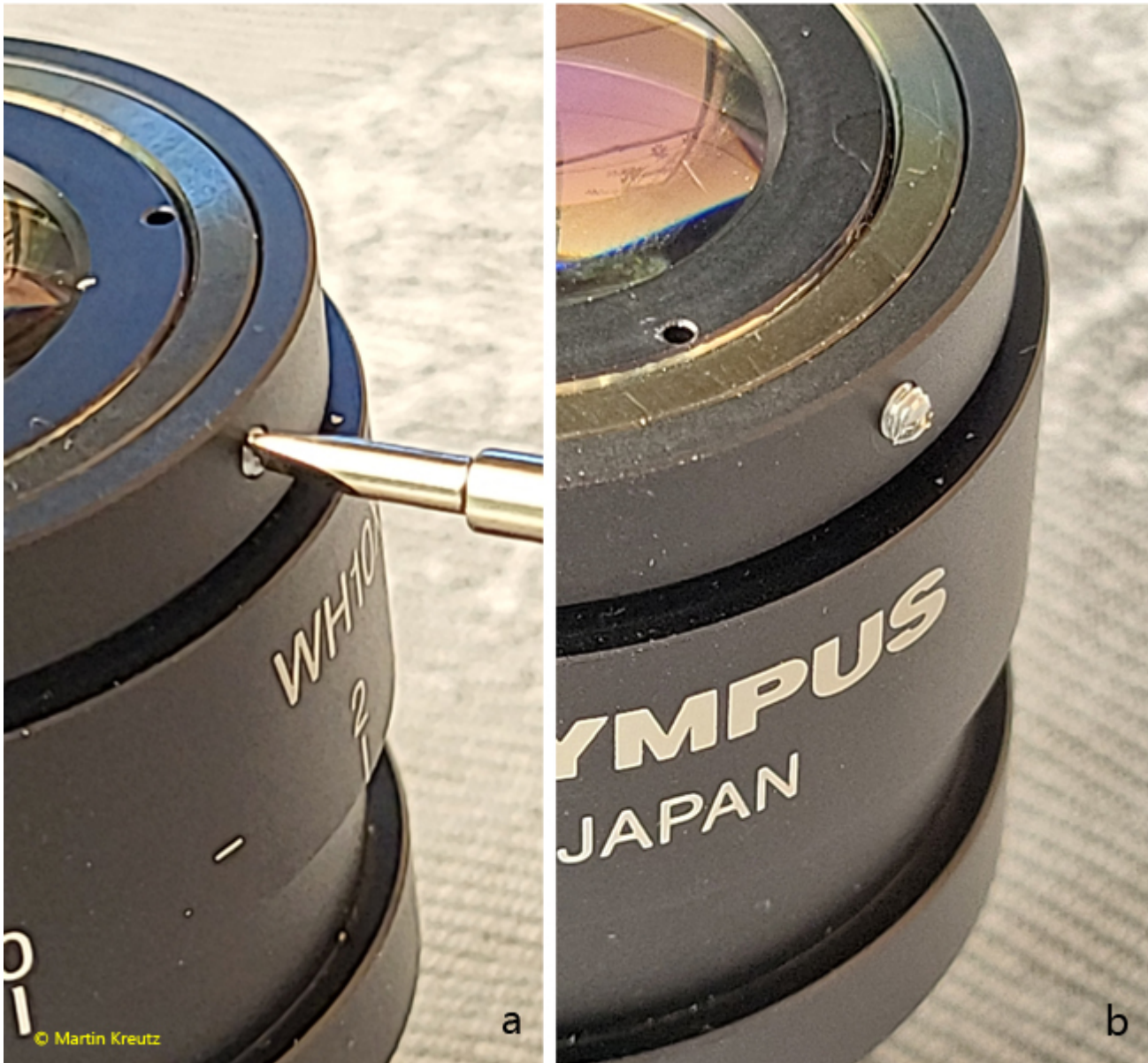
Fig. 2 a-b: Do not loosen the grub screws so much that they fall out.
