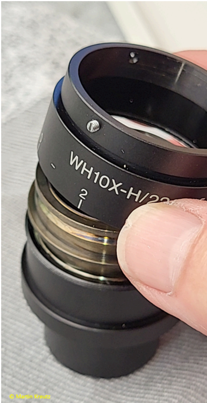
Fig. 3: Remove the upper aluminium sleeve after loosening the grub screws.
