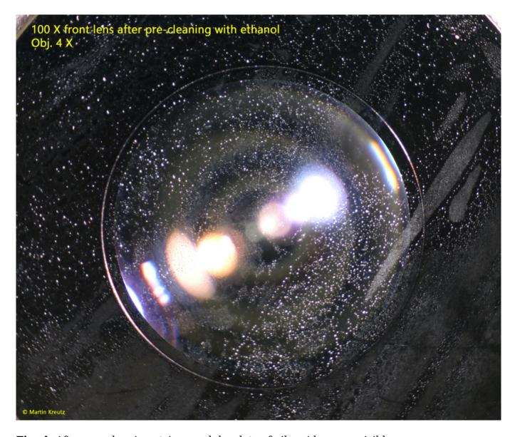
Fig. 4: After pre-cleaning stripes and droplets of oil residues are visible.
