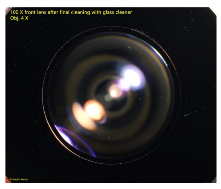
Fig. 6: After final cleaning all oil residues are removed and only tiny dust particles are visible.
