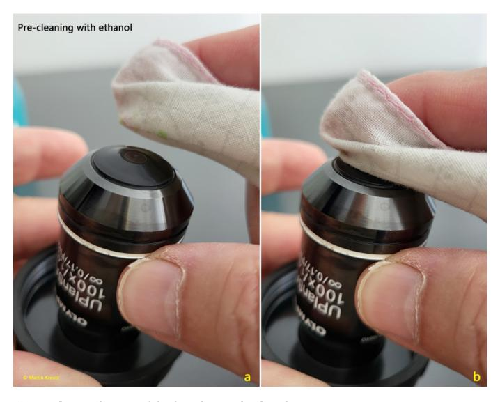
Fig. 3 a-b: Pre-cleaning of the front lens with ethanol 96%.
