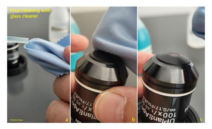
Fig. 5 a-c: Final cleaning with few drops of glass cleaner on a microfiber cloth.
