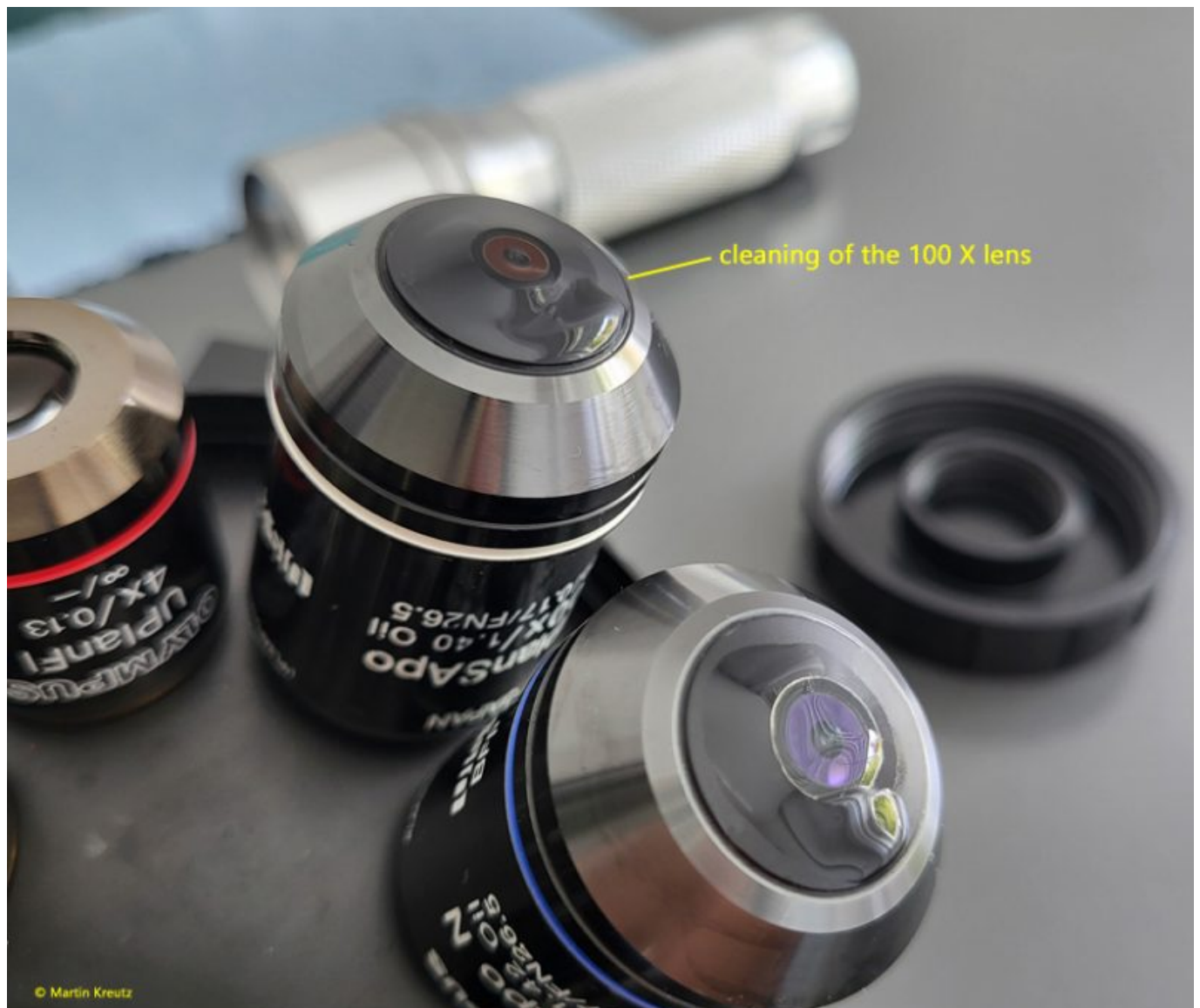
Fig. 2: In periods of about 6 months the front lens of the 100 X objective will be cleaned.
