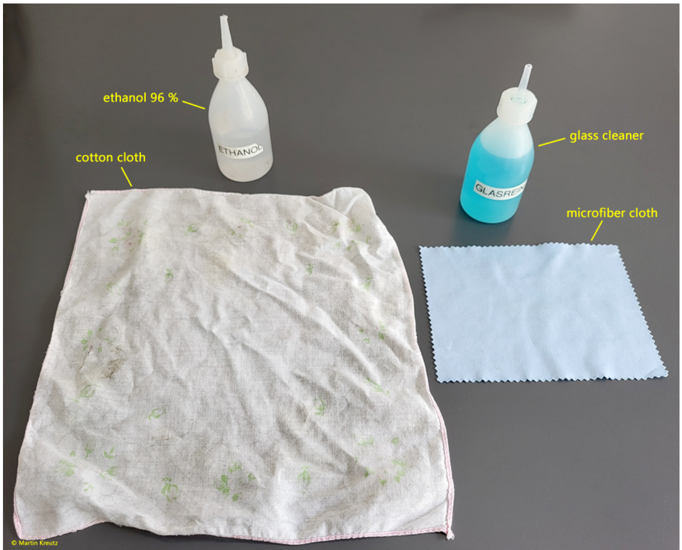
Fig. 1: The solutions and cloth needed for cleaning of immersion objectives.
