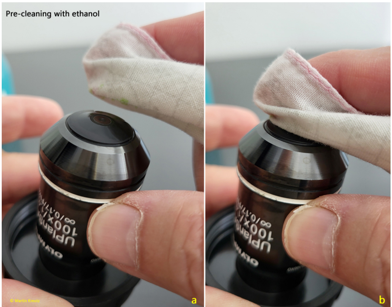
Fig. 3 a-b: Pre-cleaning of the front lens with ethanol 96%.
