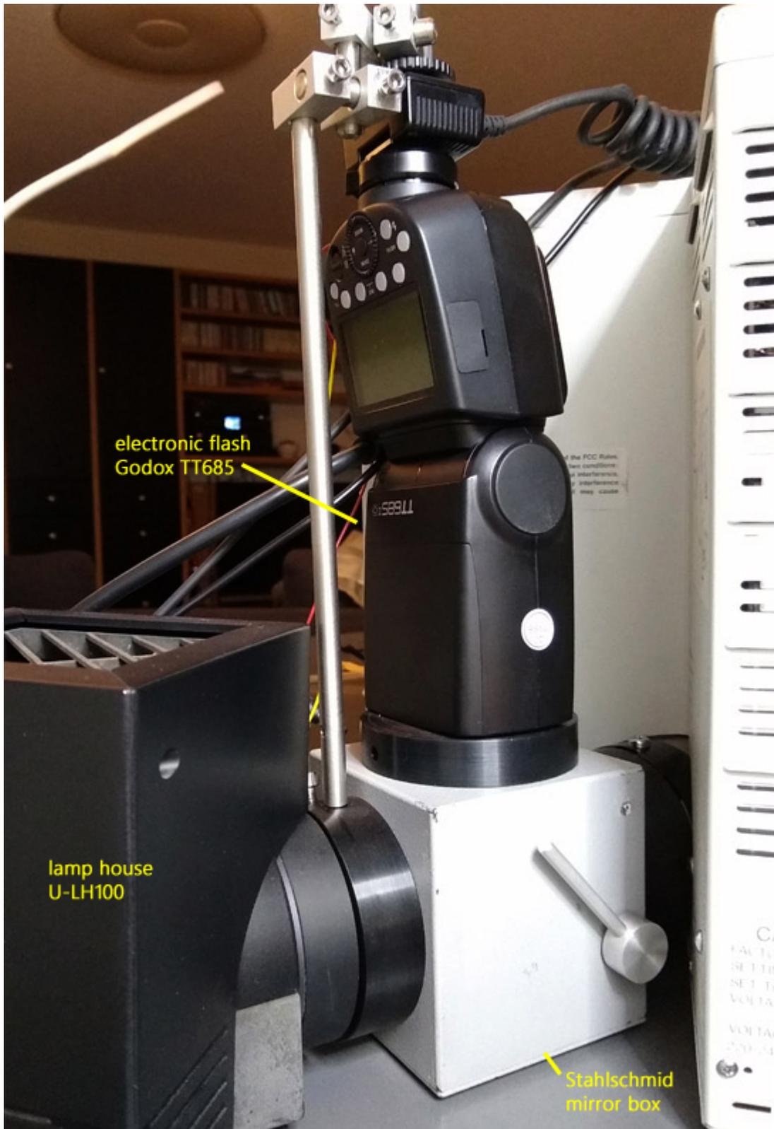
**Fig. 16:** The Godox TT685 flash positioned above the light entry window of the Stahl Schmid mirror box.
