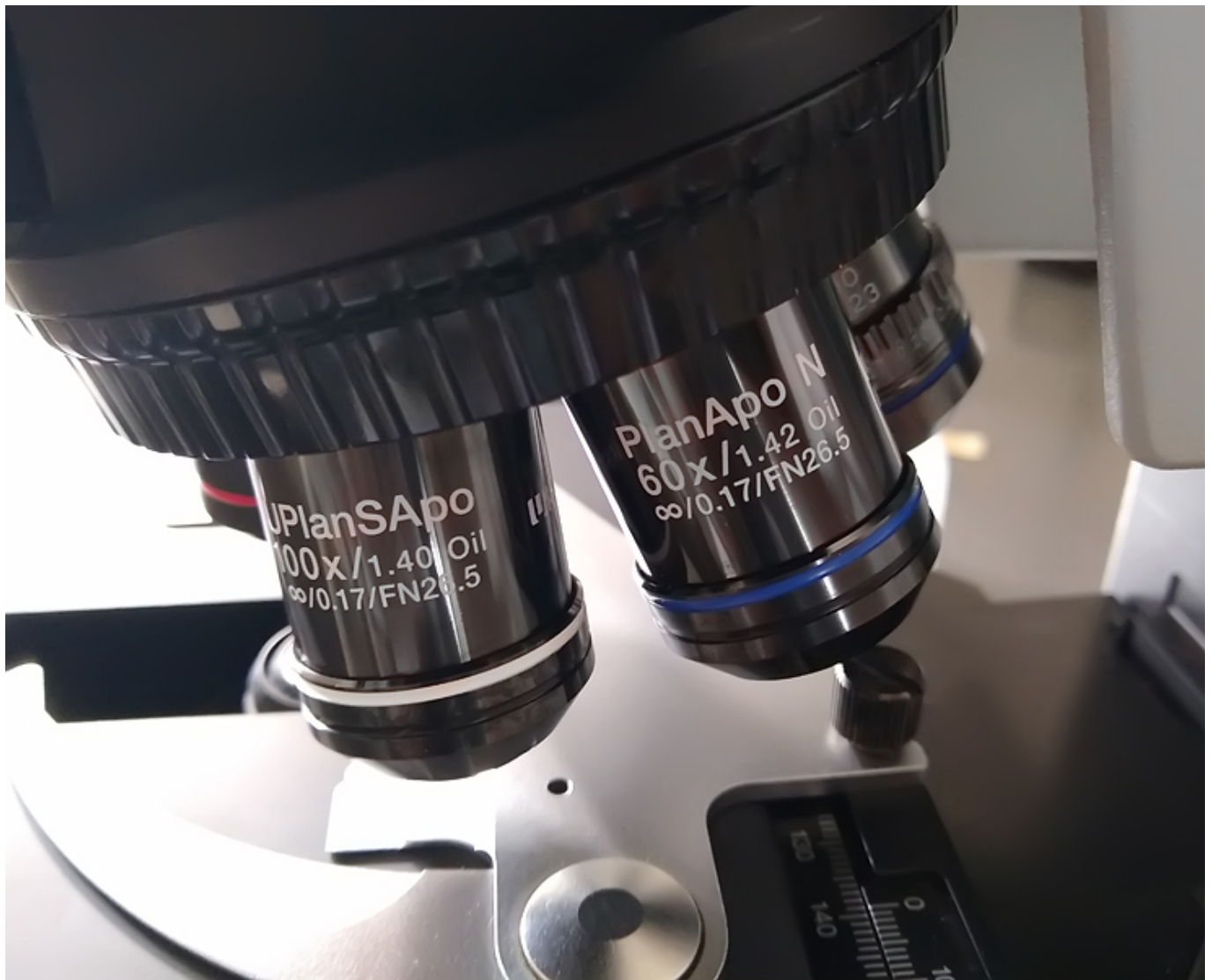
Fig. 14: The high aperture objectives Olympus PlanApo N 60X/1.42 Oil and Olympus UPlanSApo 100X/1.40 Oil provide an excellent image quality. They are my most frequently used objectives.
