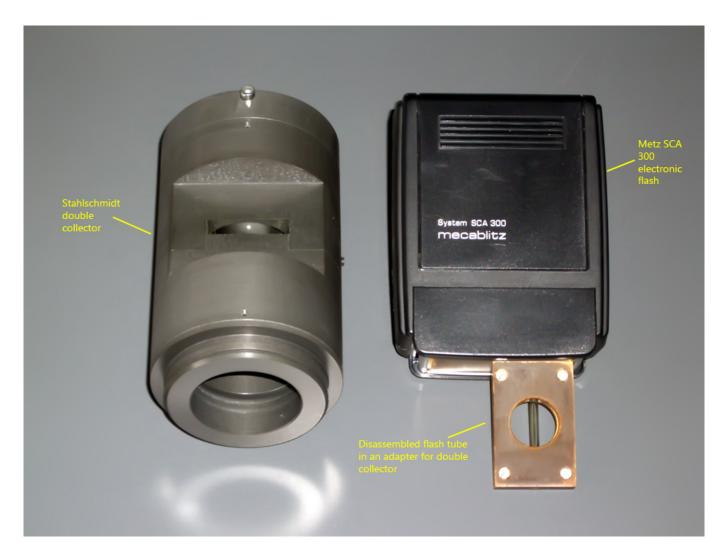
Fig. 4: The Stahlschmidt double collector and the converted Metz SCA 300 electronic flash.
