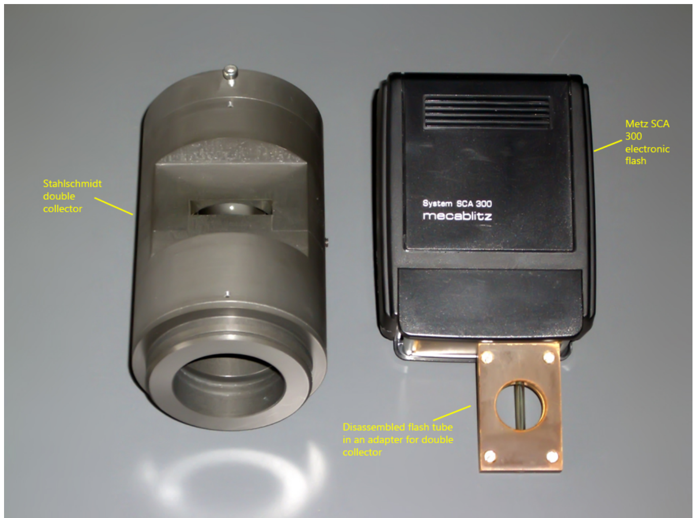
Fig. 4: The Stahlschmidt double collector and the converted Metz SCA 300 electronic flash.
