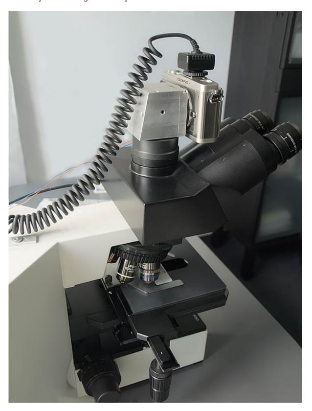
Fig. 9: The Olympus E-P1 camera connected to the Ergo-DSLR adapter.
