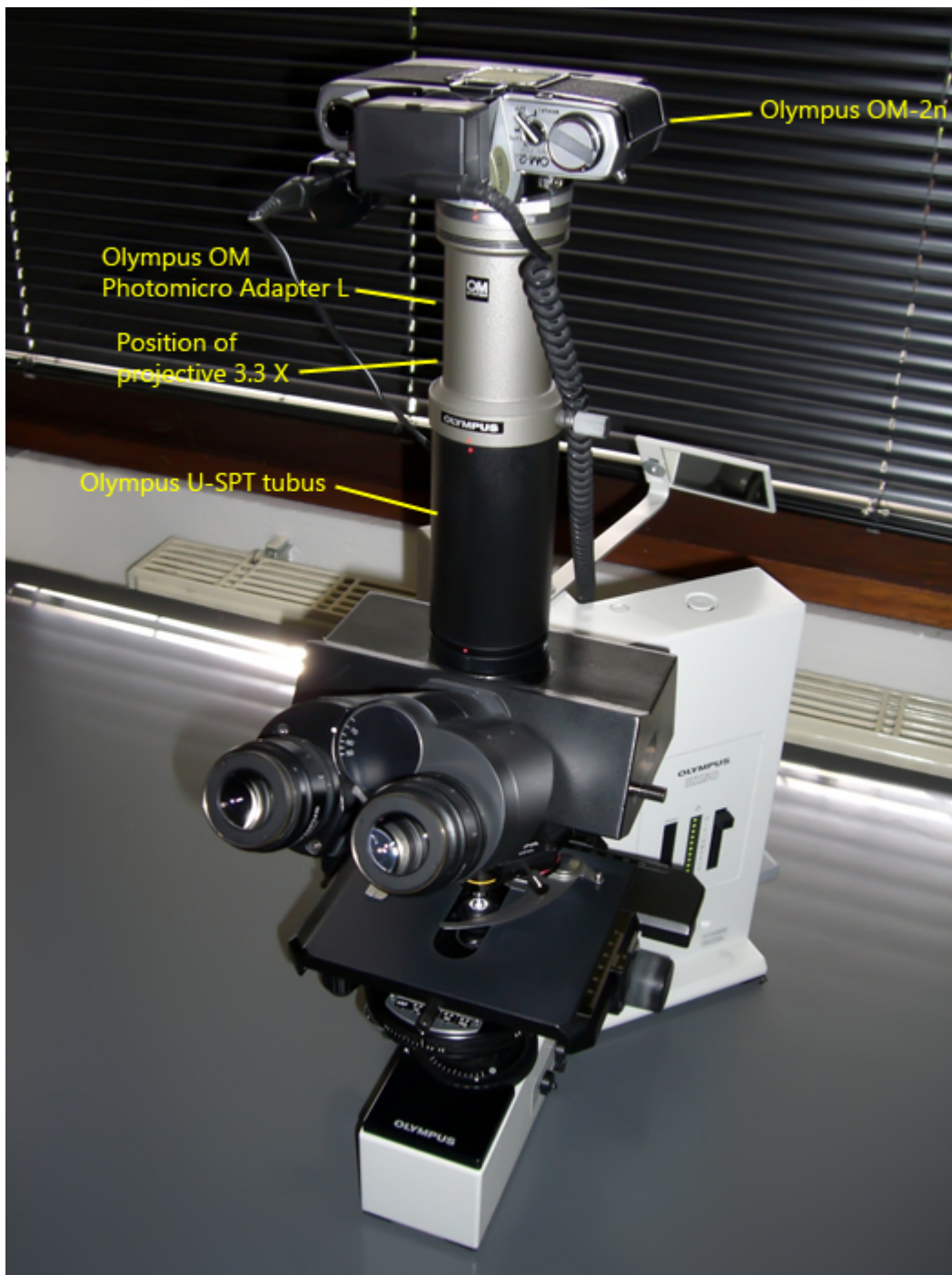
Fig. 3: Adaptation of the Olympus OM-2n camera via the Olympus U-SPT tube and the Olympus OM photomicro Adapter L. A photo eyepiece 3.3 X is inserted into the U-SPT adapter, for projection of the image onto the photo plane. June 2006.
