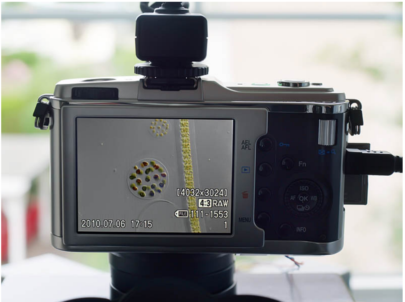
Fig. 10: Display and control panel of the adapted Olympus E-P1 camera.
