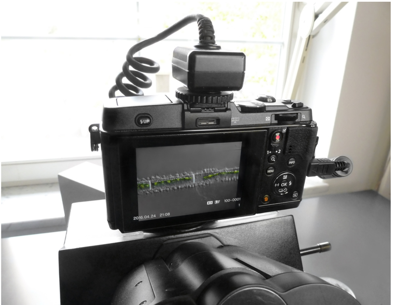
Fig. 12: View of the display and control panel of a Olympus E-P5 camera connected on to the Ergo-DSLR adapter. April 2016.
