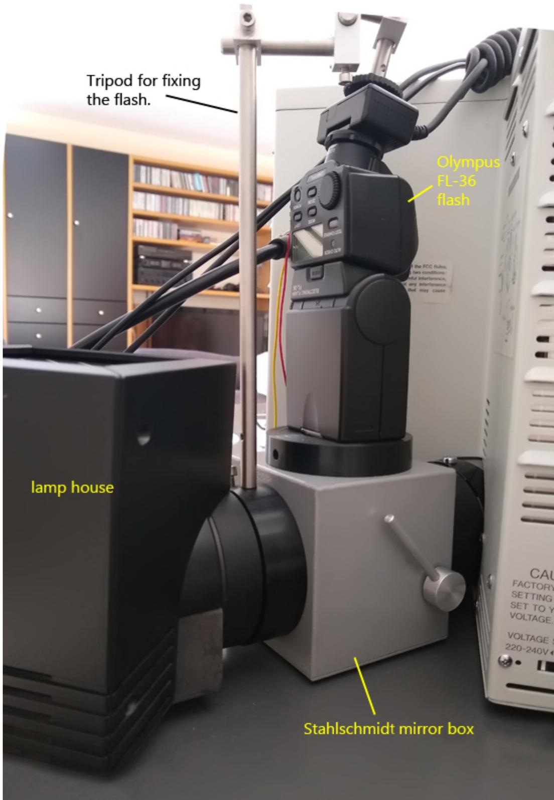
**Fig. 15:** The integrated mirror box designed and built by Jürgen Stahlschmidt with the Olympus FL-36 flash positioned above the light entry window.
