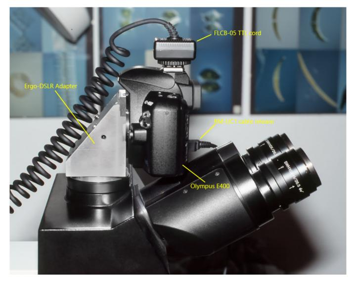
Fig. 6: The Ergo-DSLR adapter with an adapted Olympus E-400 camera. June 2007.
