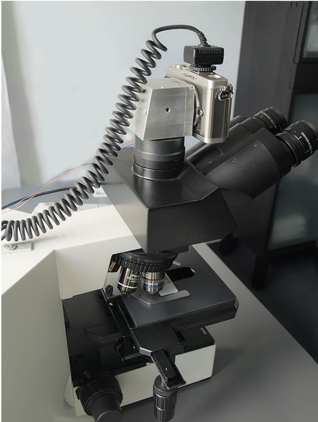
Fig. 9: The Olympus E-P1 camera connected to the Ergo-DSL adapter.
