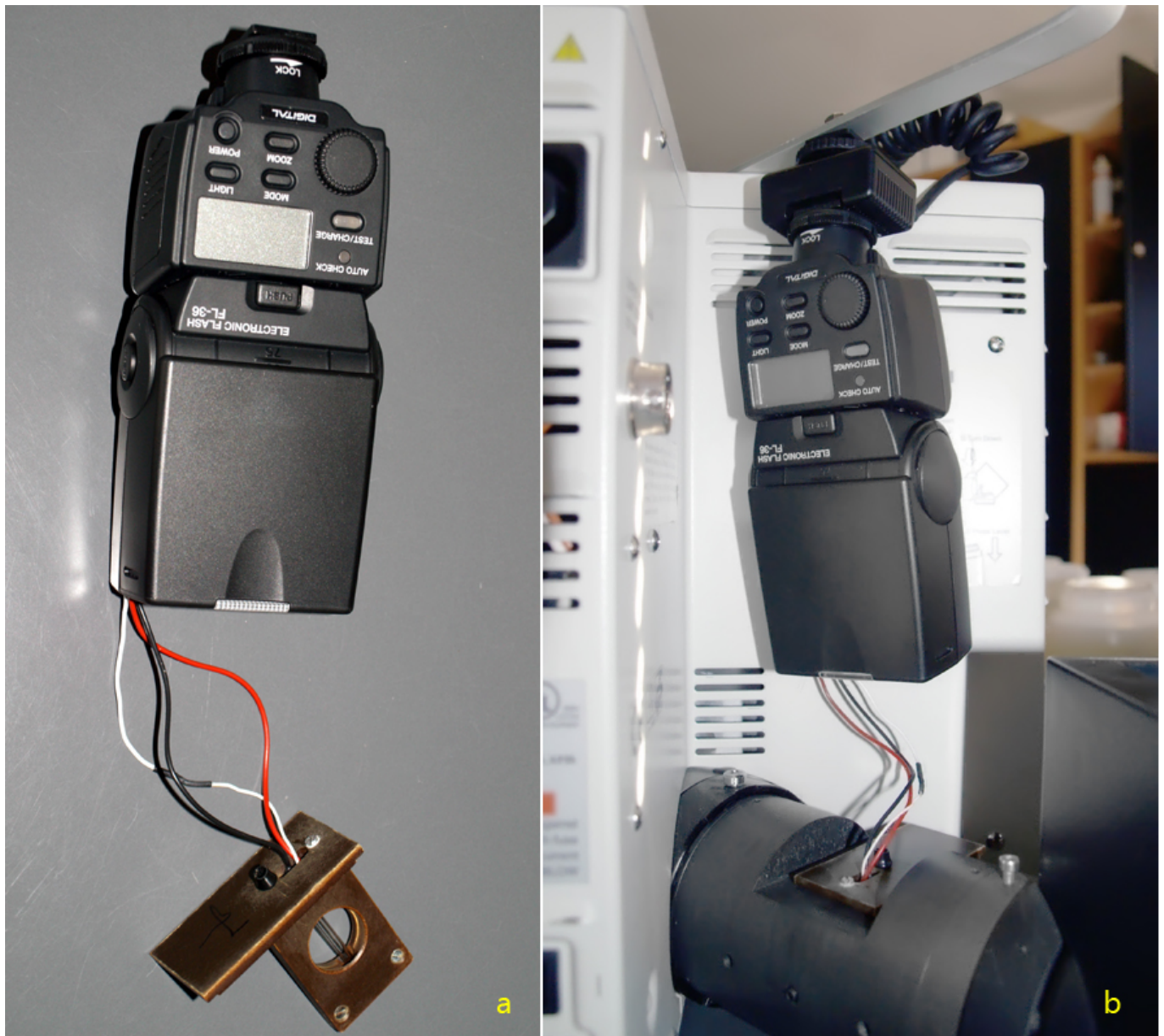
Fig. 8 a-b: The converted Olympus FL-36 flash before (a) and after (b) integration into the double collector.
