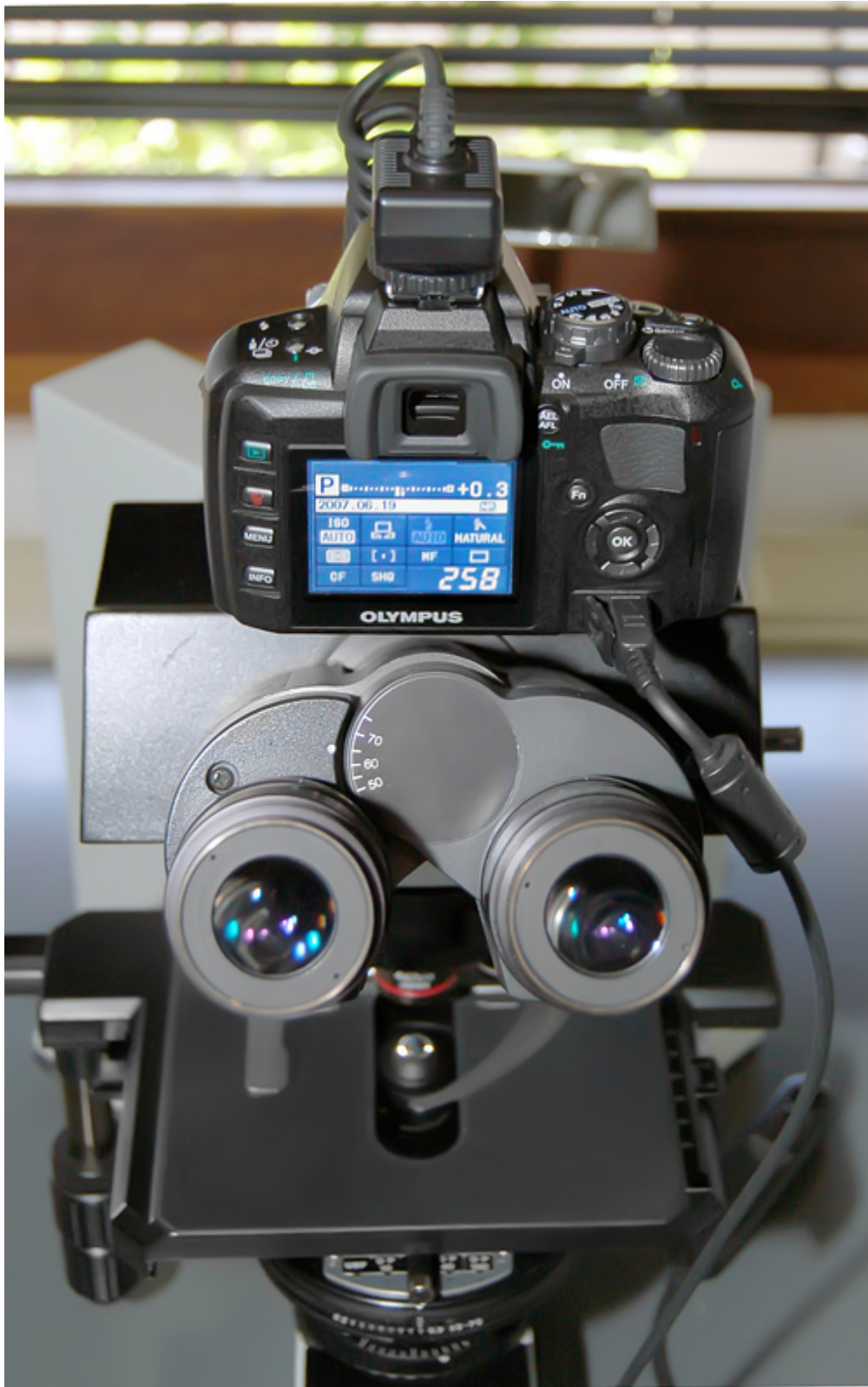
Fig. 7: The Olympus E-400 camera connected via the Ergo-DSLr adapter with the Olympus BX50. June 2007.
