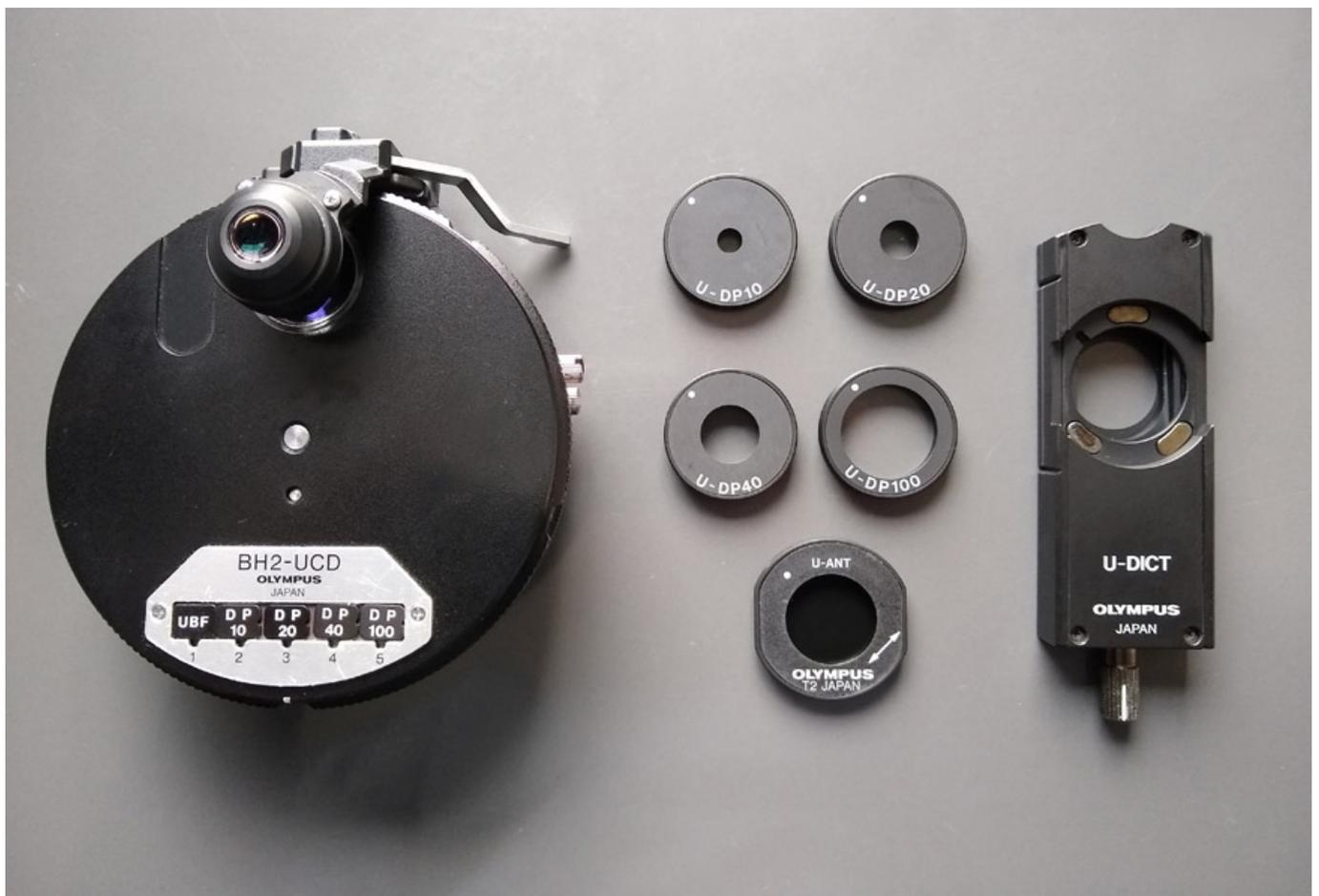
**Fig. 2:** The Olympus condensor BH2-UCD with “ordinary” DIC equipment.
