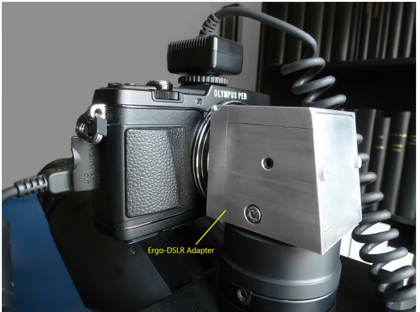
Fig. 11: The Ergo-DSLR adapter with an adapted Olympus E-P5 camera. April 2016.
