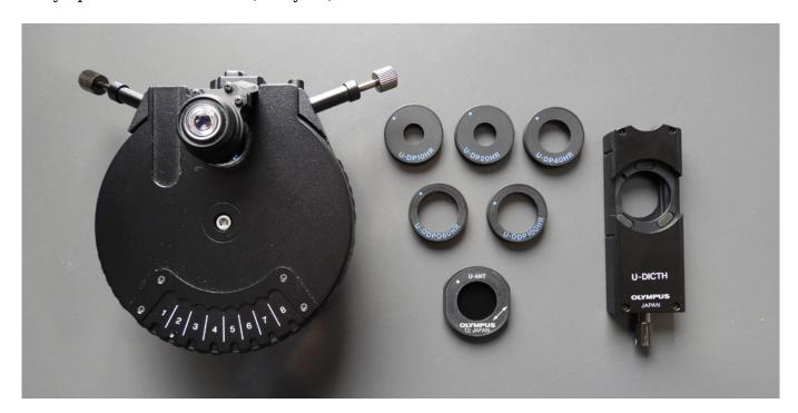
**Fig. 13:** The Olympus condensor U-UCD8 with DIC-HR equipment.
