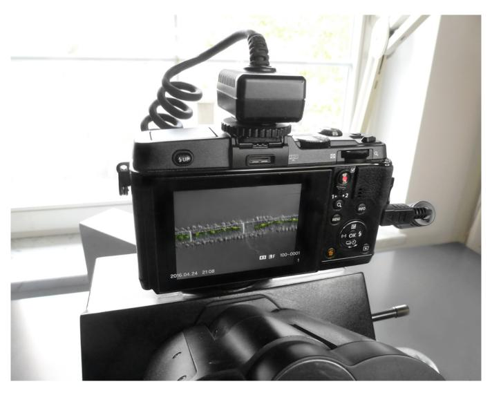
**Fig. 12:** View of the display and control panel of a Olympus E-P5 camera connected on to the Ergo-DSLR adapter. April 2016.
