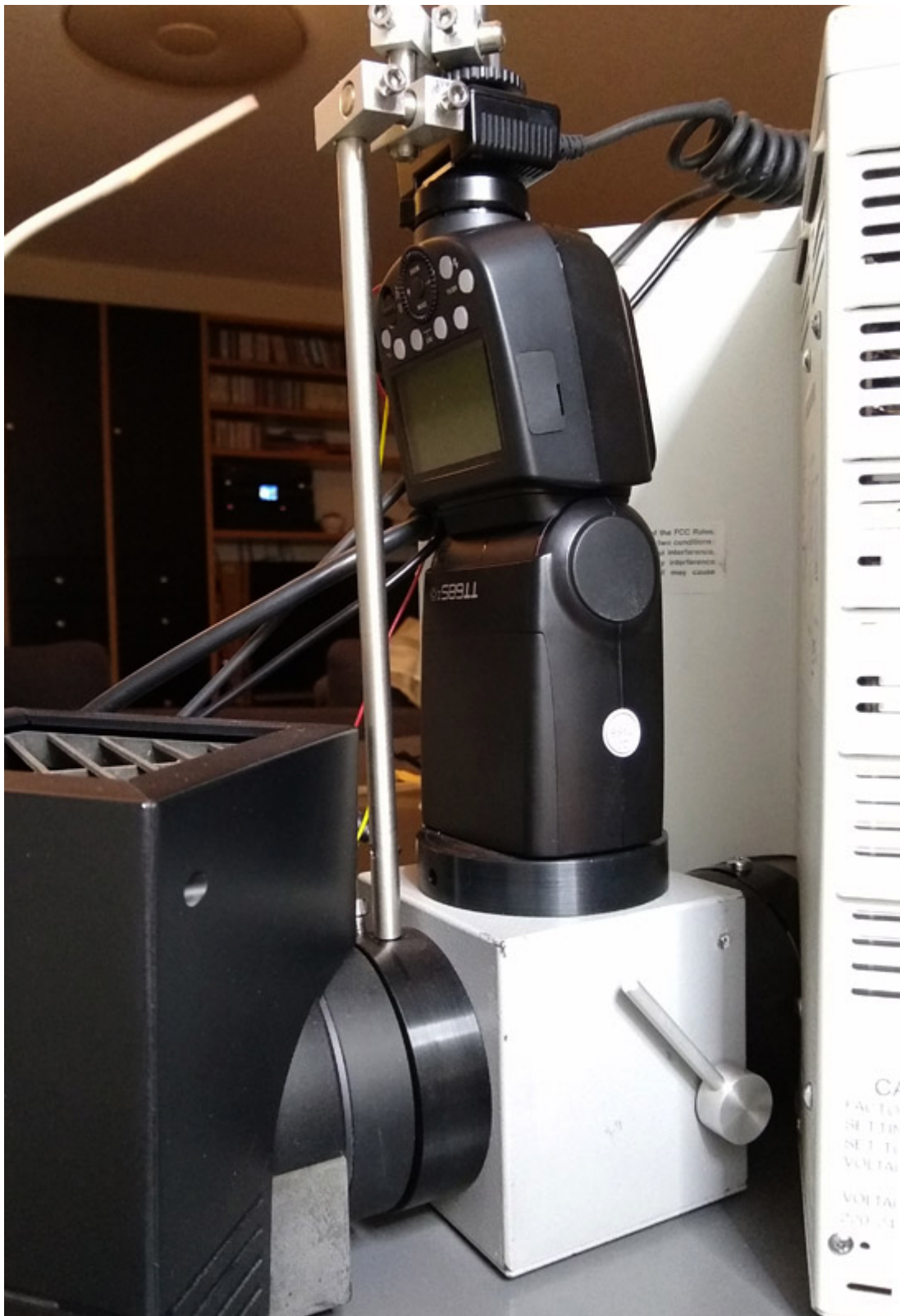
Fig. 16: The Godox TT685 flash positioned above the light entry window of the Stahlschmidt mirror box.
