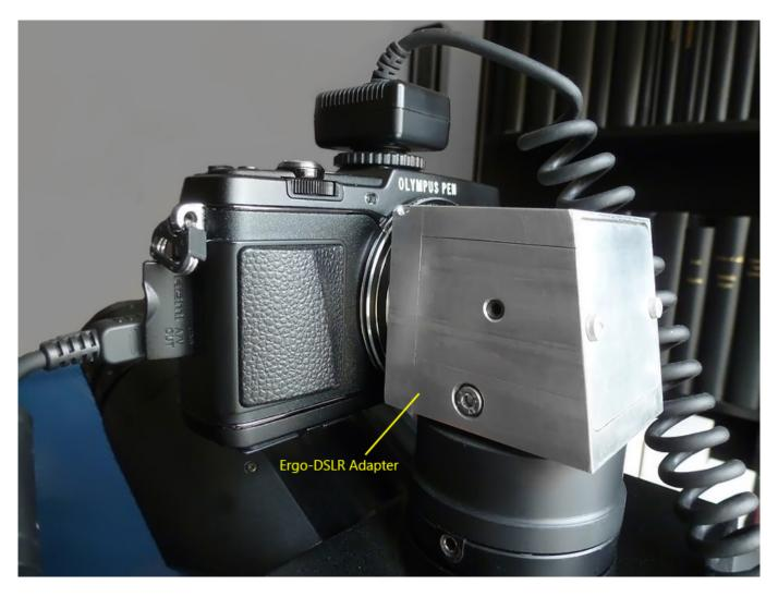
Fig. 11: The Ergo-DSLR adapter with an adapted Olympus E-P5 camera. April 2016.
