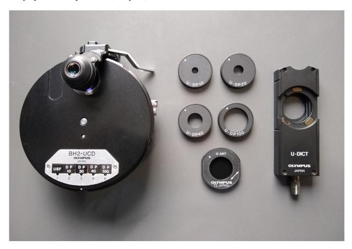
Fig. 2: The Olympus condensor BH2-UCD with "ordinary" DIC equipment.
