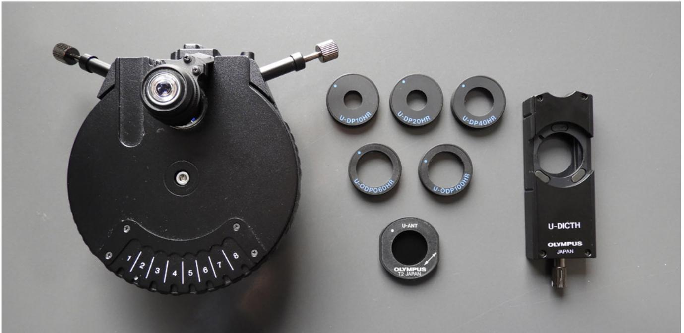
**Fig. 13:** The Olympus condenser U-UCD8 with DIC-HR equipment.
