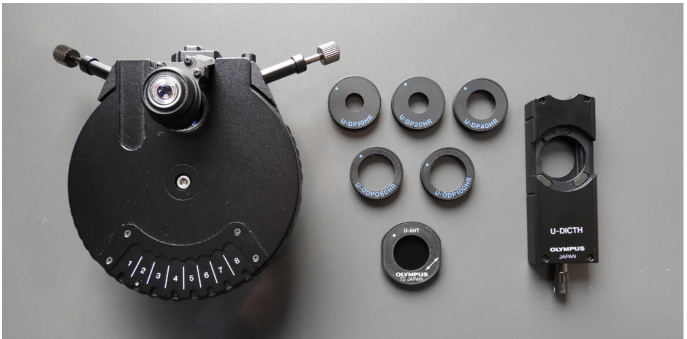
Fig. 13: The Olympus condenser U-UCD8 with DIC-HR equipment.
