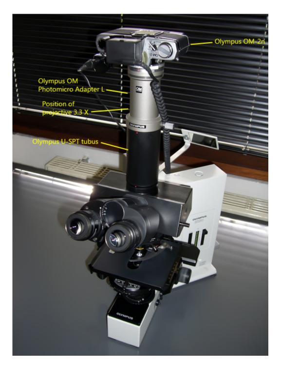
Fig. 3: Adaptation of the Olympus OM-2n camera via the Olympus U-SPT tube and the Olympus OM photomicro Adapter L. A photo eyepiece 3.3 X is inserted into the U-SPT adapter, for projection of the image onto the photo plane. June 2006.
