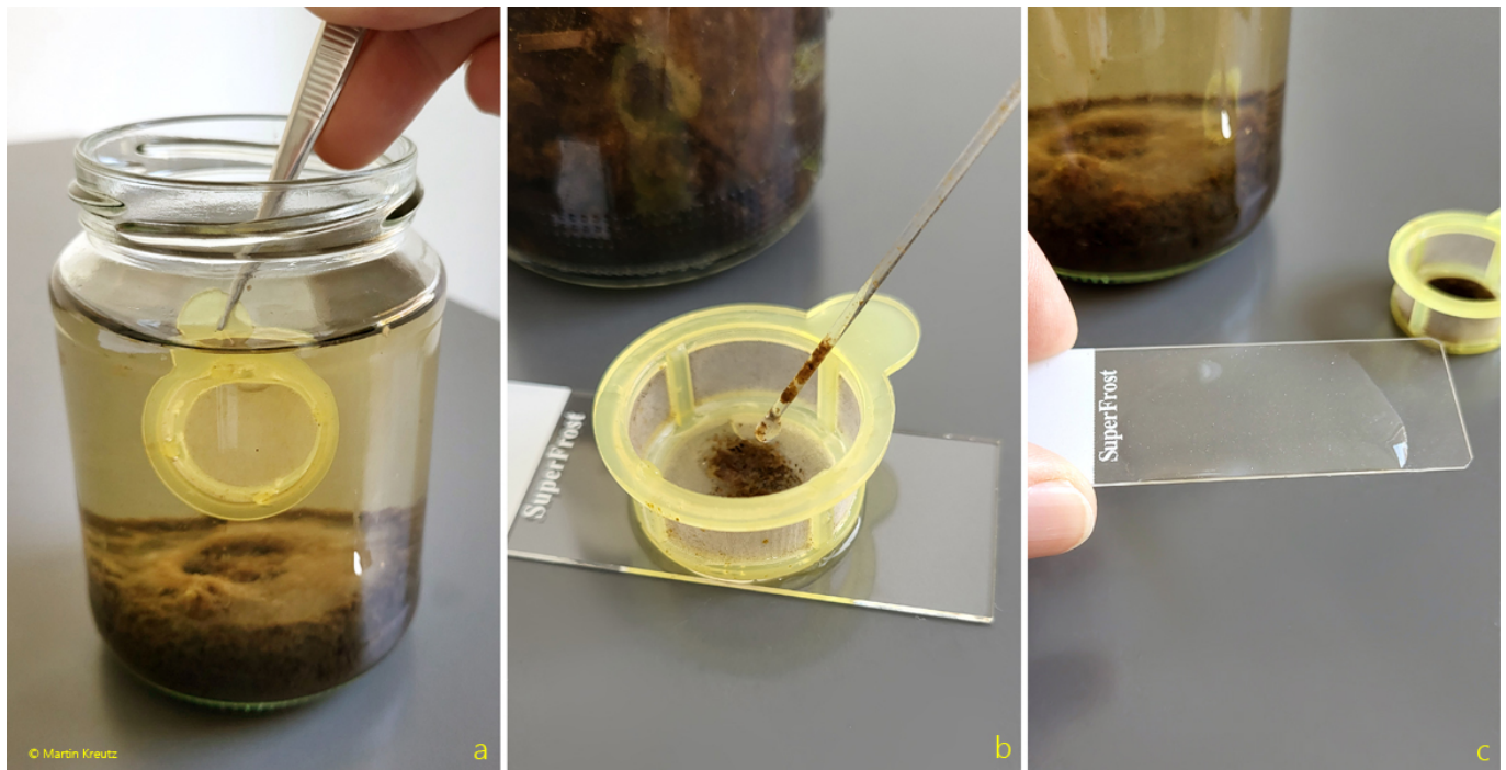
Fig. 12 a-c: Once wetted in the sample (a), the cell strainer becomes hydrophilic and allows water to pass through unimpeded (b). The sludge particles are retained (c).
