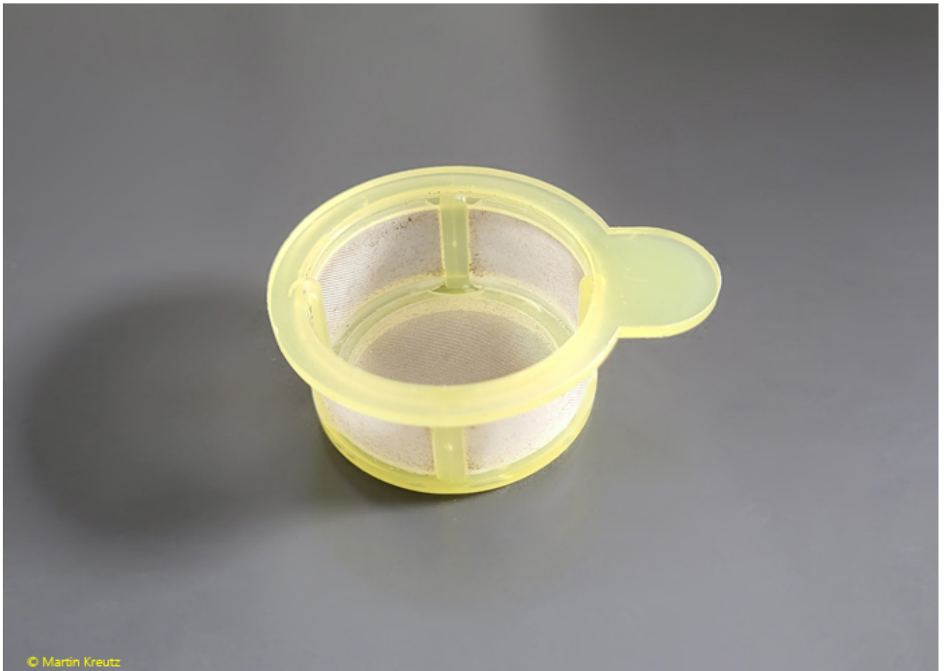
Fig. 11: A standard cell strainer with a mesh size of 100 \mu\text{m} .
