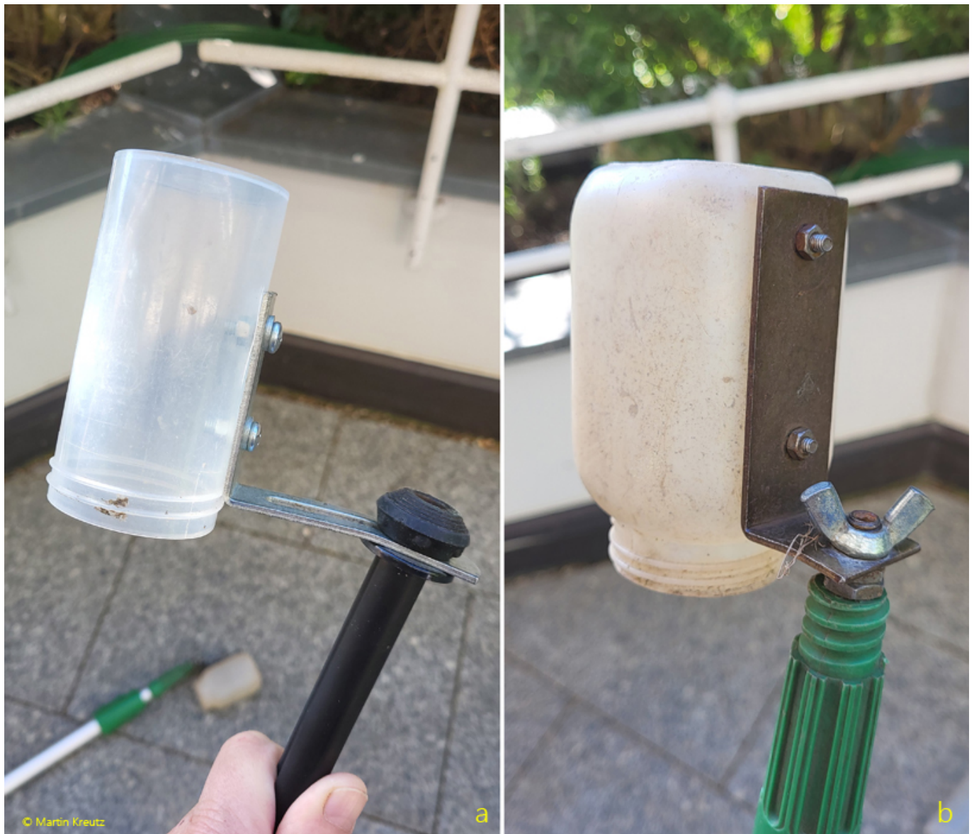
Fig. 4 a-b: The sample cups attached with the angle iron to the M8 threads of the telescopic poles.
