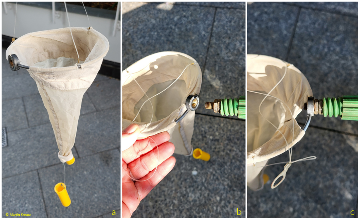
Fig. 5 a-c: The 65 µm plankton net can be attached to the telescope pole with the M8 thread.
