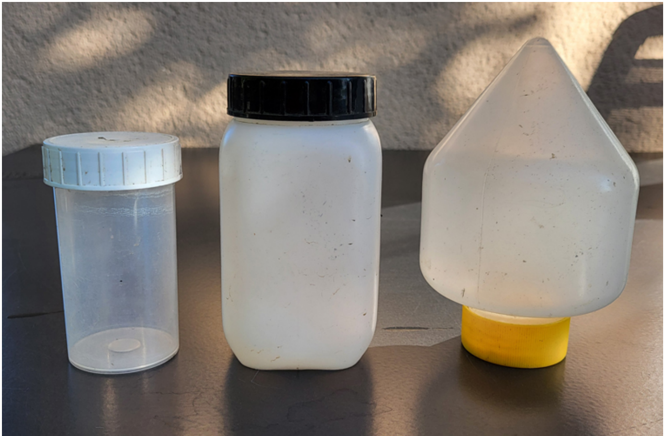
Fig. 10: The sample containers I use are made of polypropylene and have volumes of 150 ml, 400 ml, and 500 ml.
