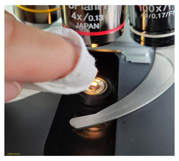
**Fig. 5:** Removal of the water from the condensor front lens with a cotton cloth.
