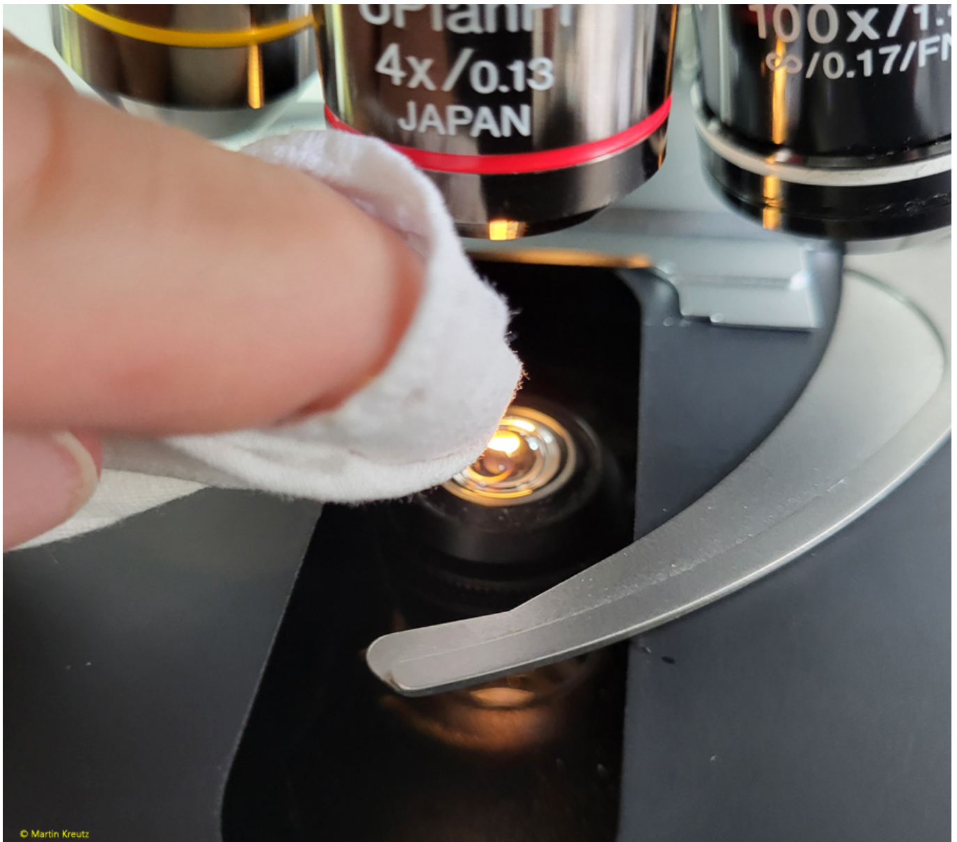
Fig. 5: Removal of the water from the condenser front lens with a cotton cloth.
