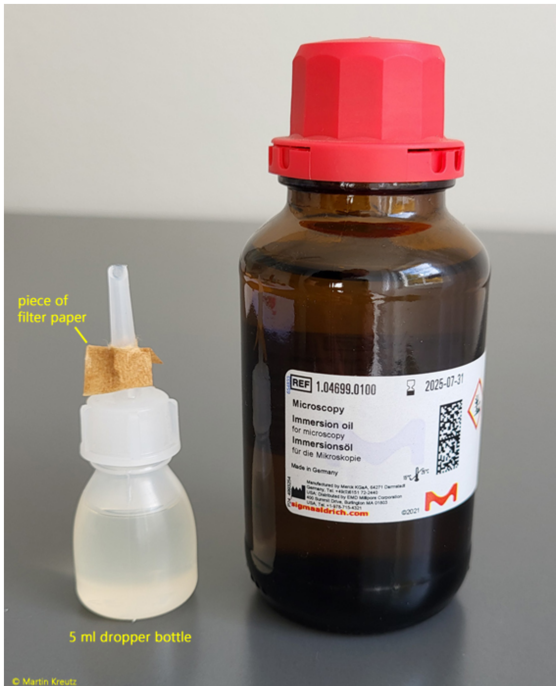
Fig. 1: The Merck immersion oil and the 5 ml dropper bottle I use to measure out the oil.
