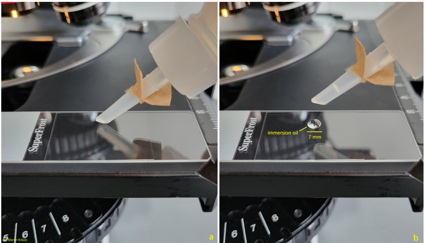
Fig. 3 a-b: Application of the immersion oil on the coverslip.
